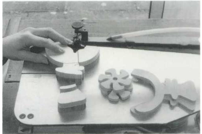
1 Having fitted the very finest blade in the scroll saw, very carefully cut the design down into its component parts. It's important that you use a new, well-tensioned blade and go at it slowly, so that each and every cut is well placed and square to the wood.
