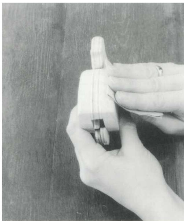
4 Rub the whole works down to a smooth finish. Close your eyes to test the finish—it's vital that every surface, edge and angle be supersmooth to the touch.
