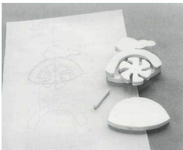
3 Test the wheels in the body cavity. They need to be an easy loose-turning fit. Note that in this test run I have the feet running in the wrong direction!
